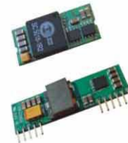
Bobcat Series 10A - 16A Output 1.3 x 0.53 x 0.32 (in) 33.0 x 13.5 x 8.1 (mm)
