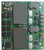
1/2 Brick Bus Converter 70A Output 2.4 x 2.28 x 0.45 (in) 60.9 x 57.9 x 11.4 (mm)
