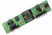
V7PC-04C Series 5V Boost at 4 A 2.5 x 0.55 x 0.35 (in) 63.5 x 14.0 x 8.9 (mm)
